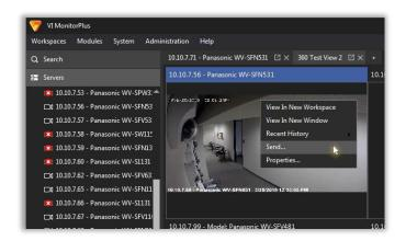
Also, the "Send" option can be invoked by right-clicking on a specific Camera streaming and opening the floating menu.
