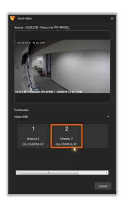
Click on the desired Video Wall monitor (orange box) to drop the selected video and to end the operation, or "Cancel" to exit.
