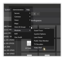
To configure Video WallPlus from VI MonitorPlus, it is necessary to *define the individual Video Wall machines* and, afterwards, the locations for each machine.
