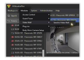
Once working on the desired Server, Camera or View, open the "Modules" option from the Main Menu, then hover on "Video Wall" and click on "Send to Video Wall".
